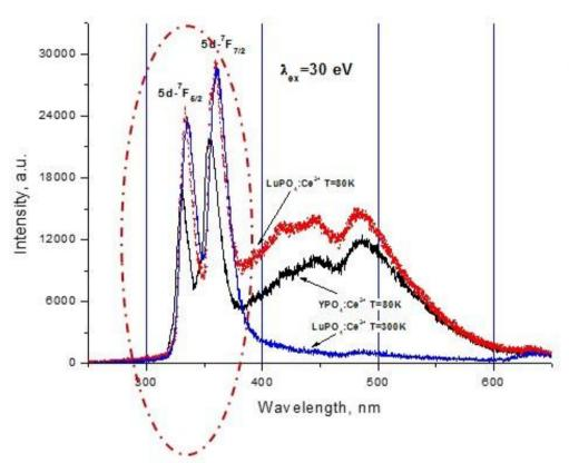
the pronounced doublet peaking at 335 and 360 nm, which is connected with 5d-4f transitions in Ce<sup>3+</sup>
