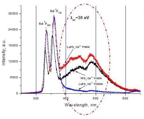
At T=80K the two broad bands were detected in 385 - 600 nm range, which are associated with defect-related emission.
